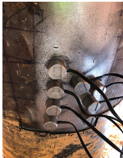
Figure 1: Dual element sensors installed permanently on identified cluster of 'low spots' on six-o'clock position of pipeline
