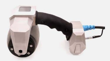
SNI introduces a new line of linear-array wheel transducers designed to improve inspection efficiency of composite materials and flat metal plate. The product's unique ergonomics facilitate operator comfort and ease-of-use when scanning large surface areas. Available in 5 different test frequencies ranging from 1 to 10 MHz, the scanning wheel can be easily swapped out.
