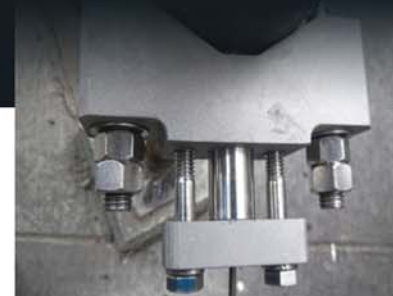
7 MHz Ultra-high-temp Delay-line: transducer and mounting clamp for continuous 500°C (932°F)
