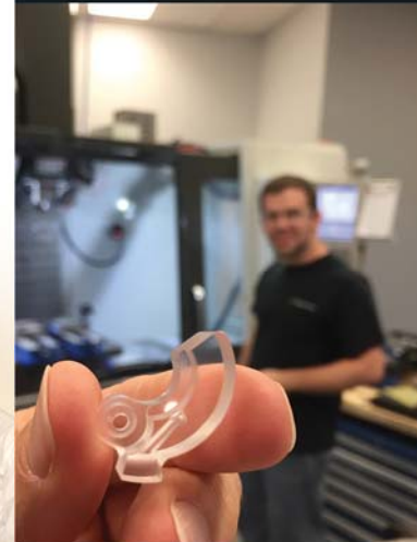
In-house CAD/CAM capabilities, including our 5-axis CNC Mill, allows for rapid prototyping of complex shapes in most engineering materials.
